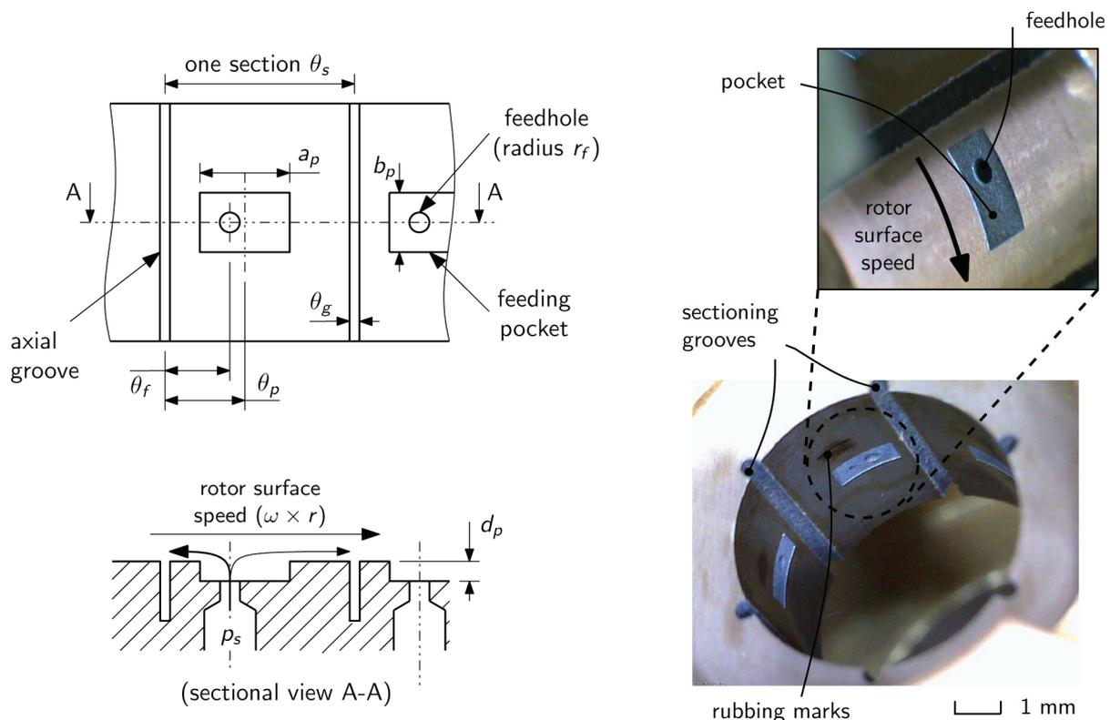
Figure 7: Schematic drawing of proposed geometry to counteract cross-coupling in the film (left); and detail view of the realised test bearing (right) [1].
