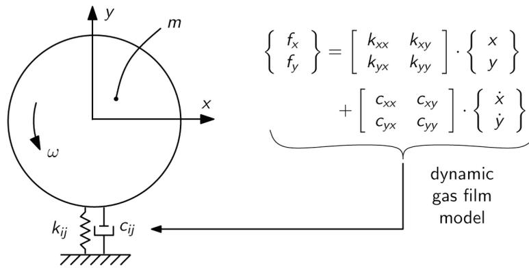
Figure 4: Dynamic model of a Jeffcott rotor-bearing system.
